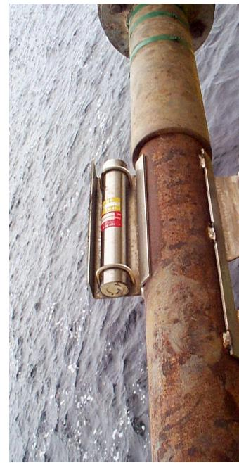
Mounting of WiSens-DA on a corer
